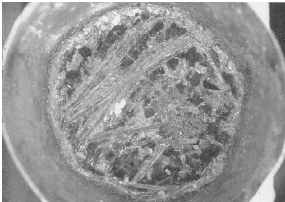
Figure 3 Rods of Pb_2MoO_5 and "discs" of MoGd_2Pb_4O_{10} at the surface of the melt in a 50 cm 3 crucible.
