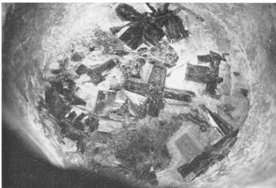
Figure 2 Er_2MoO_6 crystals on the base of a 50 cm 3 crucible.
